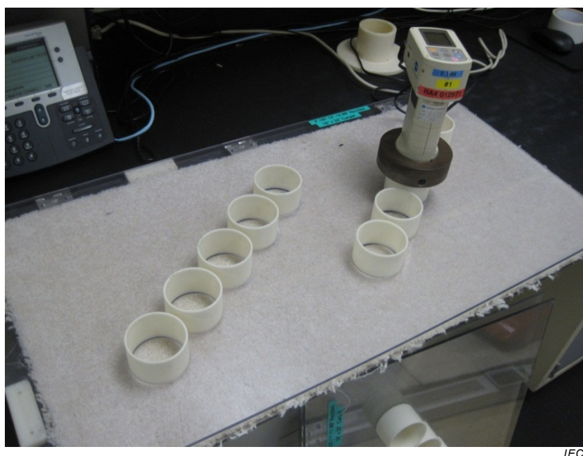
Figure 3 – Carpet colour measurement template and colorimeter
