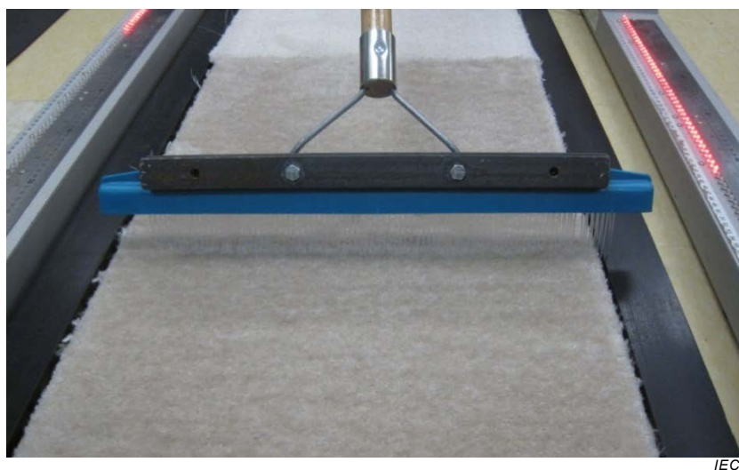
Figure 2 – Carpet grooming tool with weight
