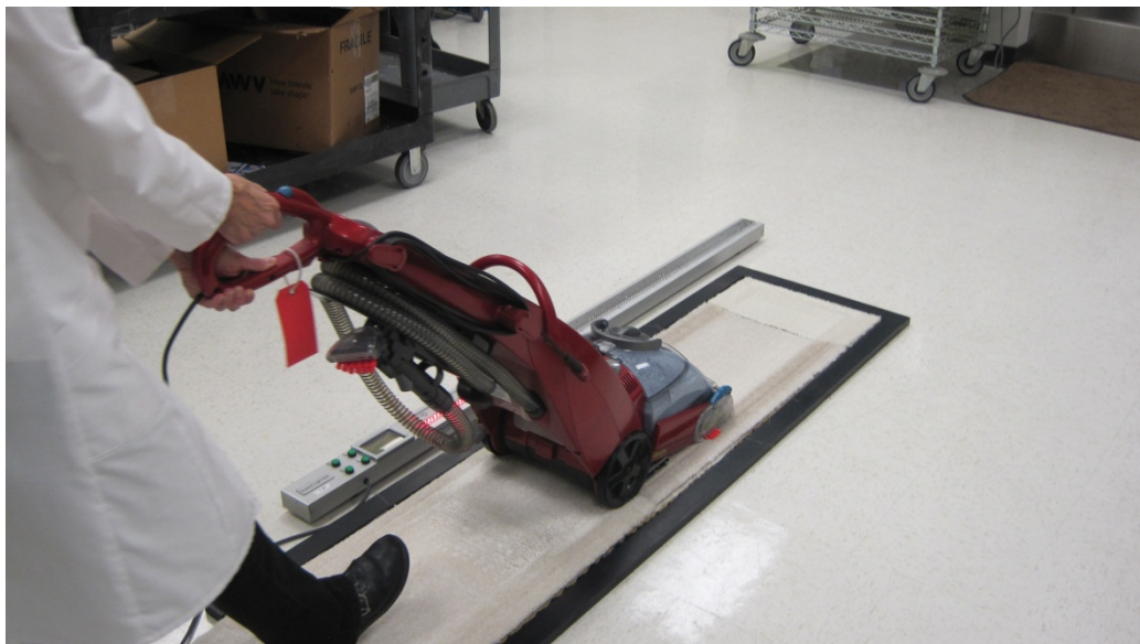
Figure 5 – Carpet cleaning template with stroke pace setting device
